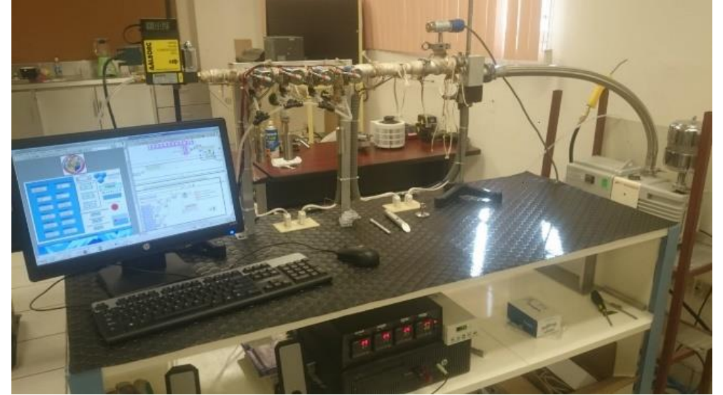
Figure 5 ALD reactor complete.
